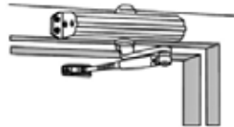
TOP JAMB INSTALLATION CLOSER IS INSTALLED ON FRAME ON PUSH SIDE OF DOOR
